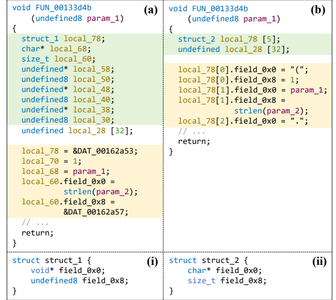
Figure 2: Motivating example that inspired the design of TYPEFORGE. (a) shows the decompiled code after retyping local_78 as struct_1 (i), while (b) shows it retyped as an array of struct_2 (ii) in the same function.
